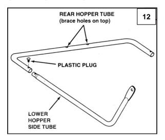
5. *(Figure 13)* Place the assembled lower hopper tubes into the bottom of the hopper bag
